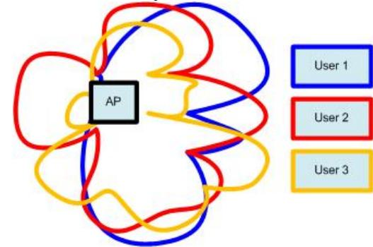
**Null-steering:** To send data to user 1, the AP forms a strong beam toward user 1, shown as the top-right lobe of the blue curve. At the same time the AP minimizes the energy for user 1 in the direction of user 2 and user 3. This is called "null steering" and is shown as the blue notches. Same logic applies to red and yellow beams.
